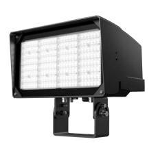
Available in two sizes, wattage packages range from 75W - 300W so that it can meet various applications. TFL comes with field-adjustable color temperature and power option as well as smart control like photocell. It's also available with various mounting options, including slipfitter mount, Yoke mount, and wall mount for flexible installations. IP66 rated.
